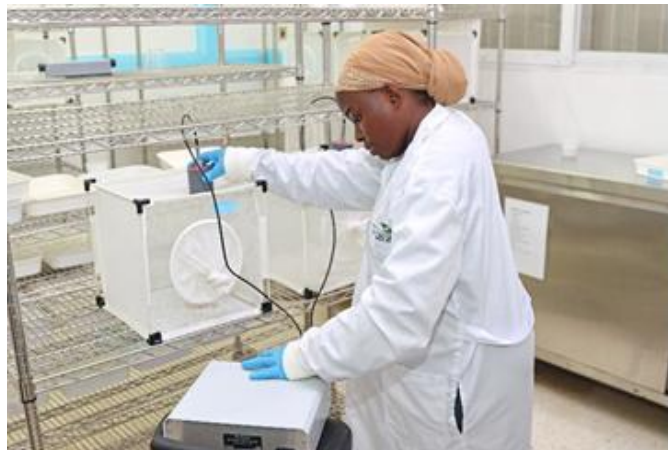
Staff setting up the Hemotek feeding system (a laboratory equipment designed for the controlled and regulated feeding of mosquitoes).
